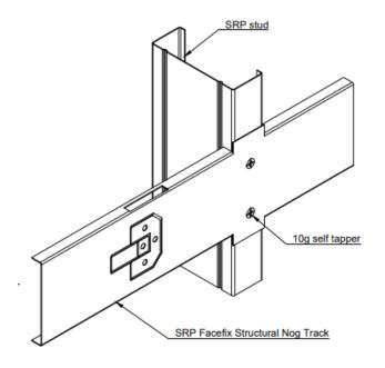
if nog centers change or an extra nog is required the legs may be snipped and folded to accomodate a stud wherever required
